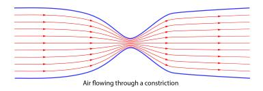
When gases flow faster the pressure within them falls and there is less pressure exerted by the gas on the walls around it. In practice this means the airway narrows even further making the situation worse.
